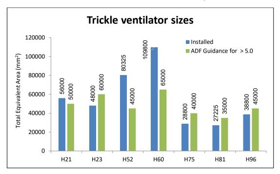
Figure 16: trickle ventilator sizes: installed vs ADF recommendations for System 1 homes
