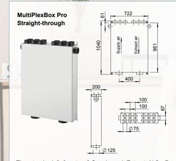
The standard 2x6 sets of Supply and Extract AirflexPro connections are orientated to give straight through duct connections. 1x extra port for supply and extract is located on the side of the unit. These are facilitated by knockout points. Compact design with easy installation and maintenance. Please see above image for the individual dimensions. Unit supplied with two inspection covers, one on each side enabling the unit to be left or right handed.
