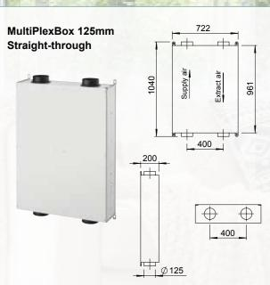
Standard 4x 125mm Ports are placed at the top and bottom of the item to give straight through duct connections. Compact design with easy installation and maintenance. Please see above image for the individual dimensions. Unit supplied with two inspection covers, one on each side enabling the unit to be left or right handed.
