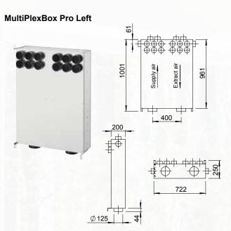
The standard 2x6 Supply and Extract AirflexPro connections are orientated 90 degrees to the main body. 1x extra port for supply and extract is located on the side of the unit. These are facilitated by knockout points. Compact design with easy installation and maintenance. Please see above image for the individual dimensions. The supply air to the dwelling is on the left hand side in this unit as you look at the unit.
