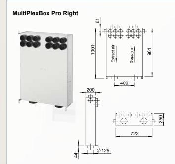
The standard 2x6 Supply and Extract AirflexPro connections are orientated 90 degrees to the main body. 1x extra port for supply and extract is located on the side of the unit. These are facilitated by knockout points. Compact design with easy installation and maintenance. Please see above image for the individual dimensions. The supply air to the dwelling is on the right hand side in this unit as you look at the unit.
